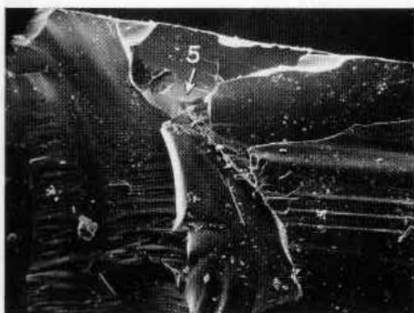
Figure 4. Photograph of a large fracture surface of the Slocum stone. (Photo taken with the Scanning Electron Microscope (SEM) at 53x.)
